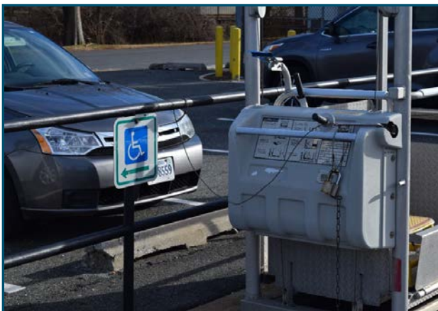
Mobile lift at northbound platform at the station in Aberdeen
