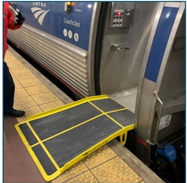
Bridge plate to span the gap between the platform and train for mobility devices at 30th Street Station, Philadelphia
